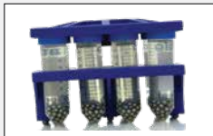
BigFlex™ Adapter 8 x 50 mL tubes
