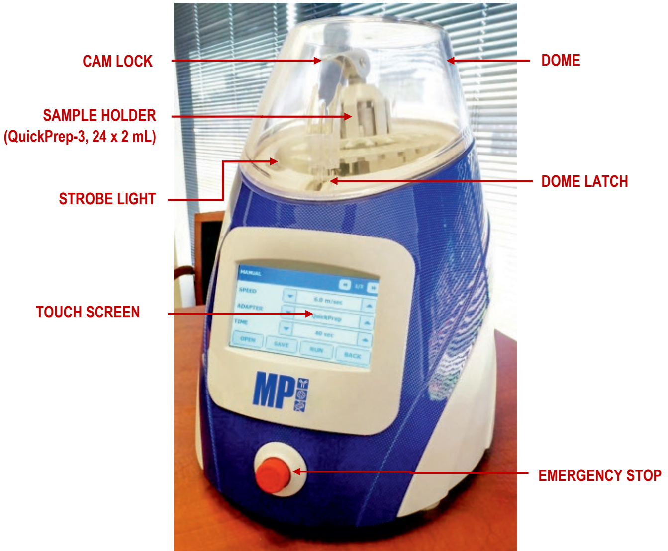
Figure I-1: Major Components of the FastPrep-24™ 5G (Front View)
